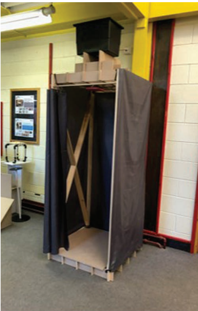
Above: Sophie's final A Level project, a flatpack shower for use in developing countries, which includes a carbon filtration system to purify the water for drinking. The waste water is recycled for use in agriculture.
